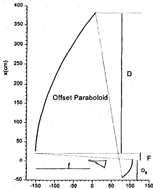
Figure 1. Dual reflector configuration
