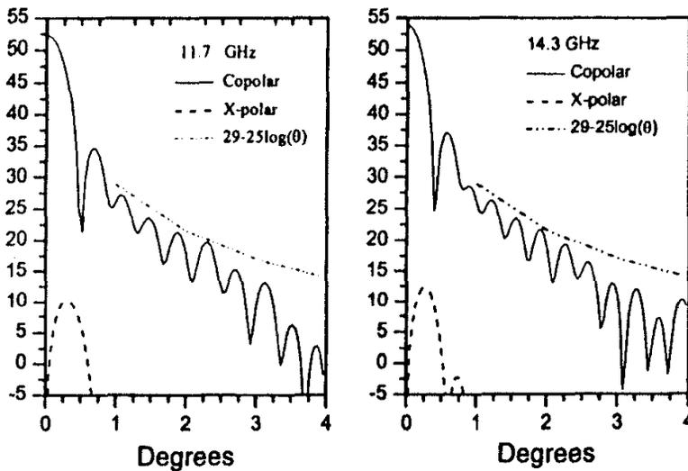
Figura 3 - Antenna radiation patterns in the asymmetry plane
