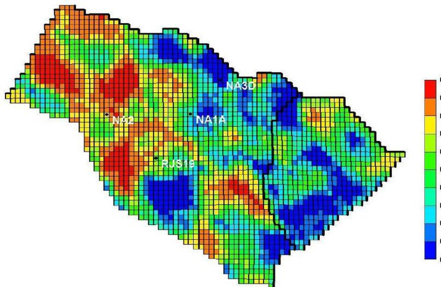
Figure 5.12: Porosity map of UNISIM-I showing position of the perforated wells and the location of the fault.
