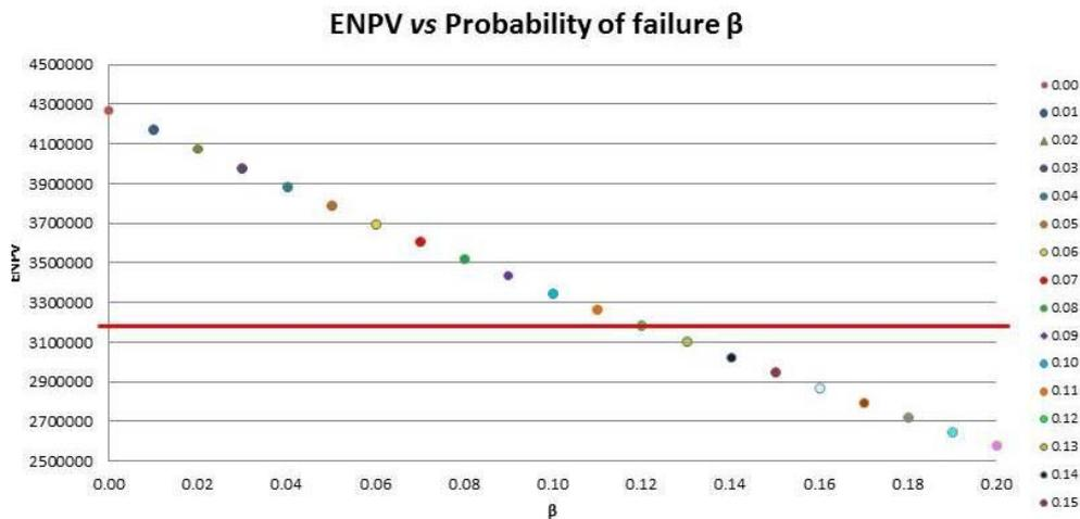
Figure 5.11: ENPV behavior when all valves fail with different probability of failure beta considering alpha constant equal 0.1 and that valve fail fully open or fully closed position. The red line represent the limit of ENPV obtained by the base case without failure
