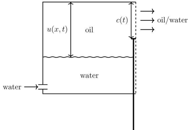
Figure 5.28: Schematic of continuous tank model
