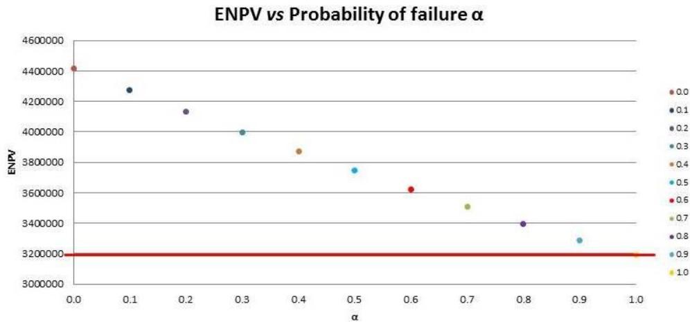
Figure 5.10: ENPV behavior when all valves fail with different probability of failure alpha considering that valve fail on the previous settings. The red line represent the limit of ENPV obtained by the base case without consider failure.
