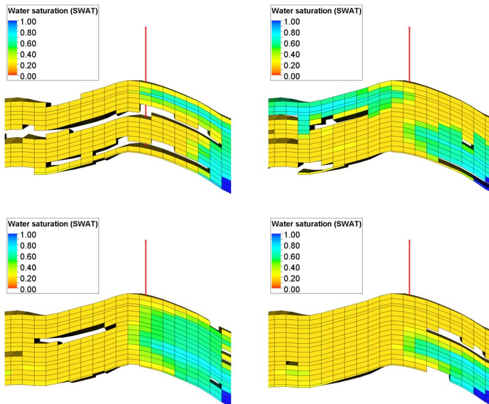
Figure 5.17: Multiple realizations of the water saturation after 6 years of production with conventional completions.
