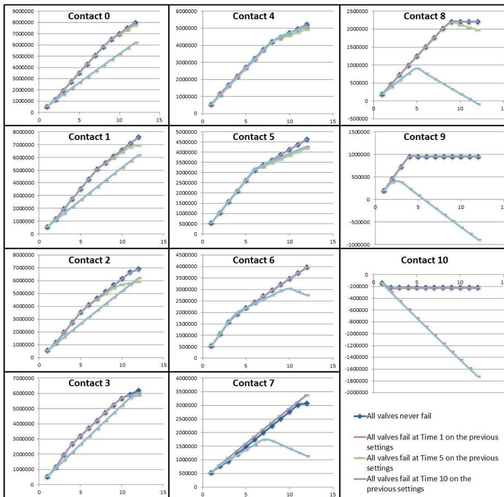
Figure 5.7: ENPV behavior when all valves fail on the previous settings varying the time of failure for each uncertainty scenario.
