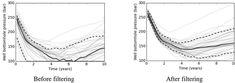
Figure 5.23: Bottomhole pressure over time in one of the wells that is considered for installation of intelligent completion.
