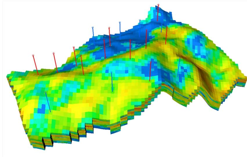
Figure 5.15.: Reservoir and well model, with producer wells in red and in water injector wells in blue.
