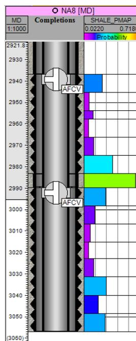
Figure 5.16 Design of a completion string, with packers at the top of the reservoir and at the level of the low permeability layer.
