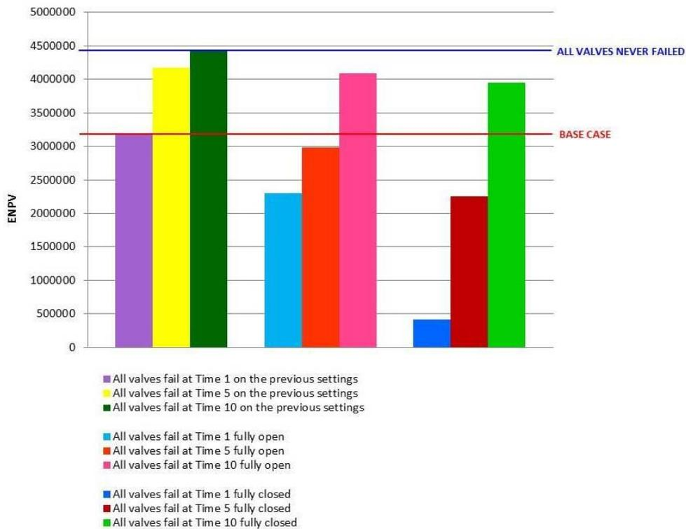
Figure 5.9: The cumulative ENPV behavior when all valves fail fully open or fully closed.
