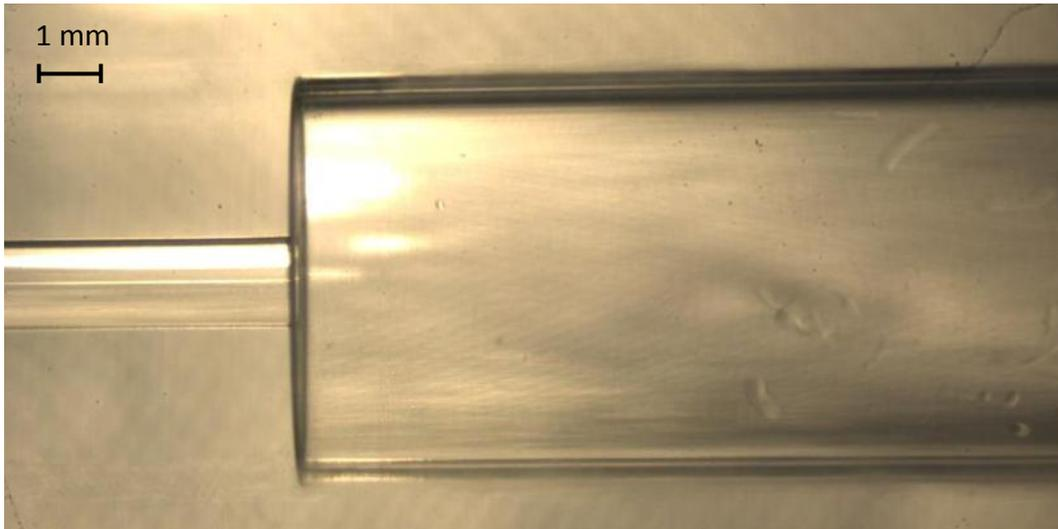
**Figure 4. 15** Droplet breakup and initial fragmentation in a low interfacial tension system (6 ms after the initial breakup).  $\mu_d = 0.0178$  Pa.s,  $\sigma = 1.97$  mN/m,  $\beta = 0.22$ , Orifice Length = 5 mm,  $T = 25$  °C.
