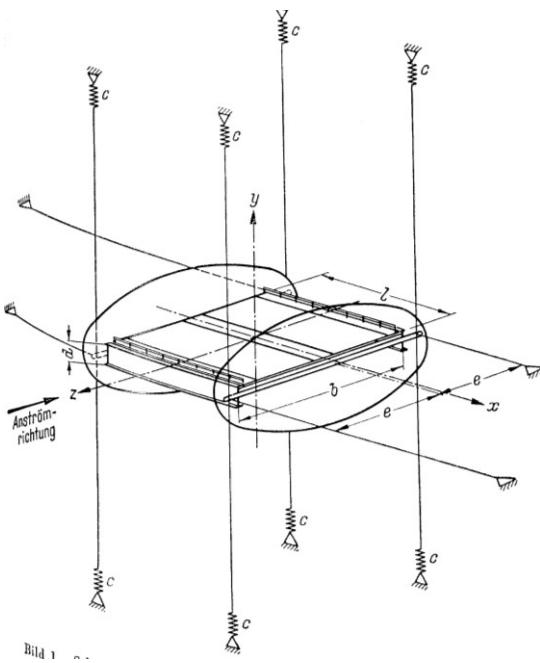
Figure A-2- Wind tunnel set up showing the suspended model under wind flow.
