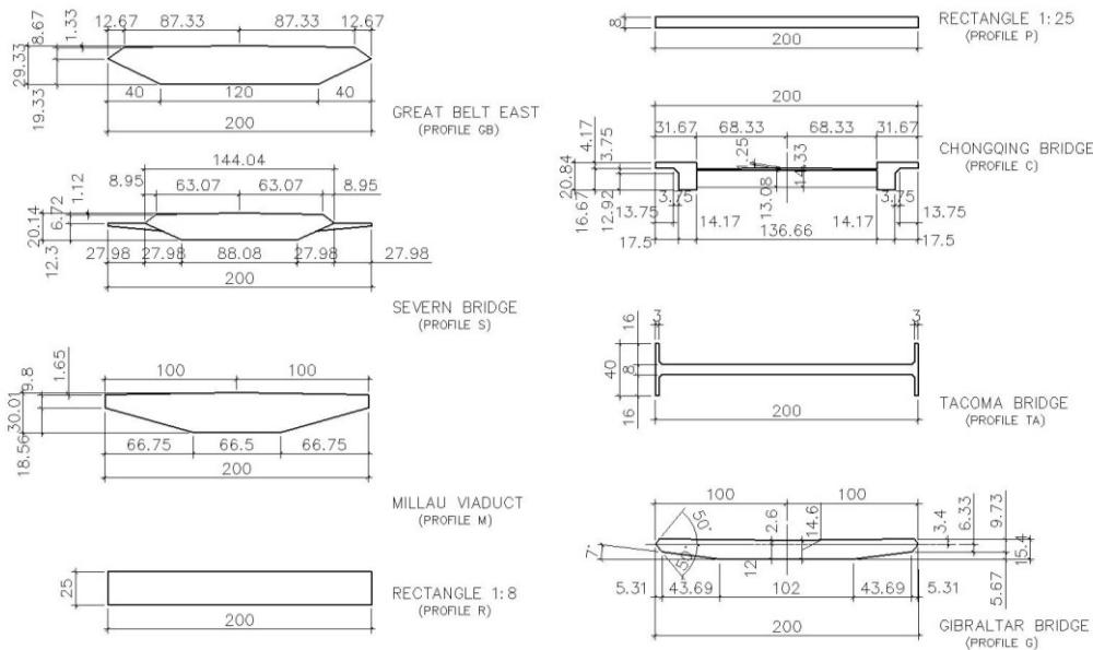
Figure D-1 - Investigated profiles of typical bridge decks.
