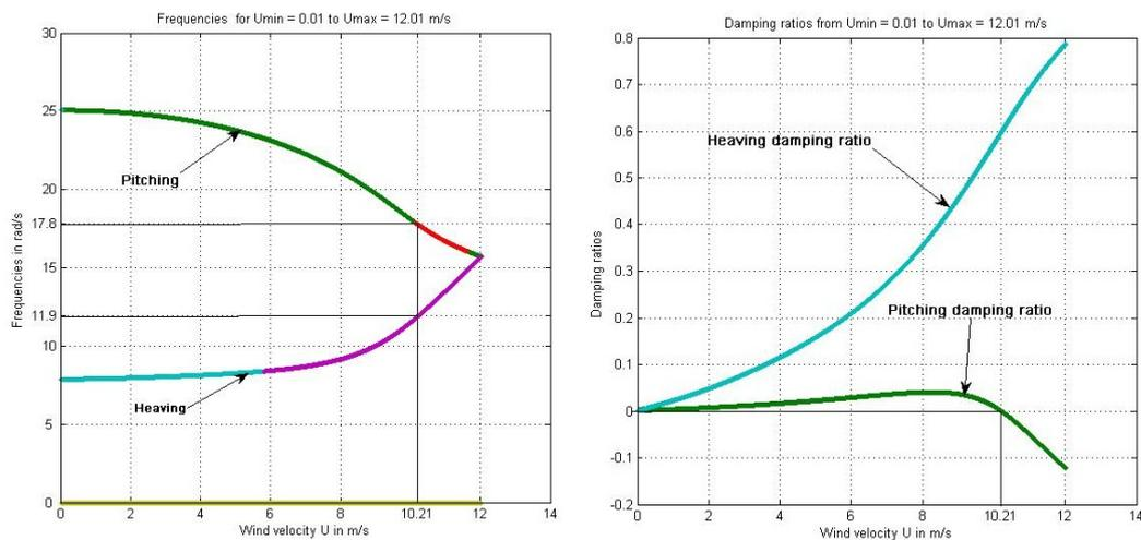
Figure 4-2 - Variation of frequencies and damping ratios versus wind velocity
