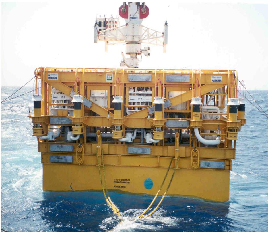
Figura 1.42 - *Manifold* UMC (*Underwater Manifold Center*)
