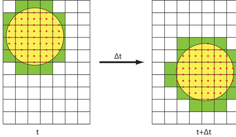
Figure 3.3: Fixed mesh at every instant of time.
