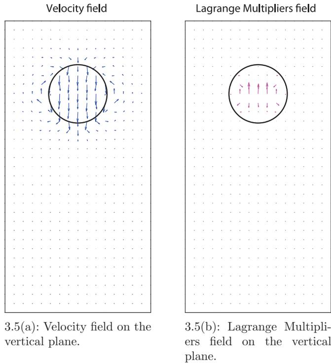
Figure 3.5: Velocity and Lagrange Multipliers fields on the plane  $z = 0$  of the 3D flow with one particle. Notice the rigid body motion inside the particle and that  $\lambda$  is zero in the fluid domain.
