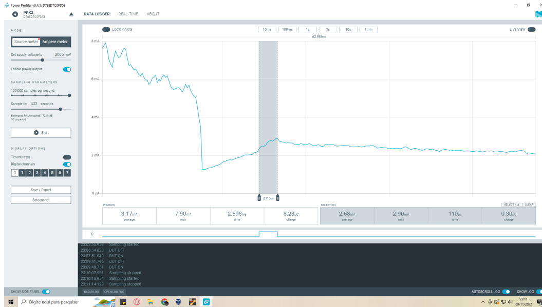
Figure 4.12: NRF Power Profiler Kit II chart. Acquisition of energy requirement of the self-adaptive procedure in the WKit BLE version.
